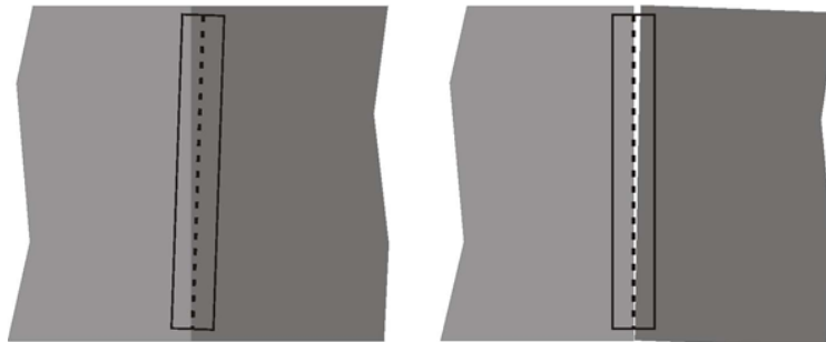
Tape not aligned with ticket junction Tickets not tightly butted
